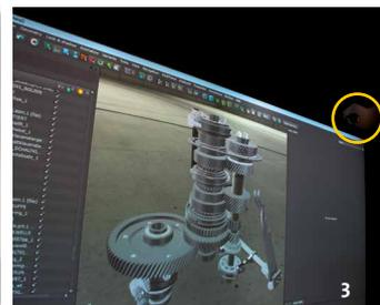
1| Media control: Via tablet PC, the display on the wall is changed to split screenmodus 2| Central remote: A cluster, consisting of four PC’s in the black rack, modifying data for projection. 3| High-End Stereoscropy: The wall with DeltaGen 10.0 software. The tracking camera for interaction with the projected model, is visible at the upper right side of the wall.
