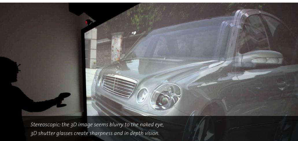
*Stereoscopic: the 3D image seems blurry to the naked eye, 3D shutter glasses create sharpness and in depth vision.*
